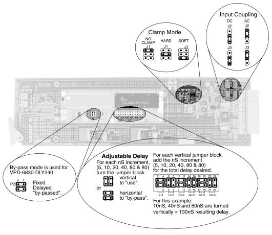
Figure 8-15. VPD-6830-DLY Series Jumper Location
